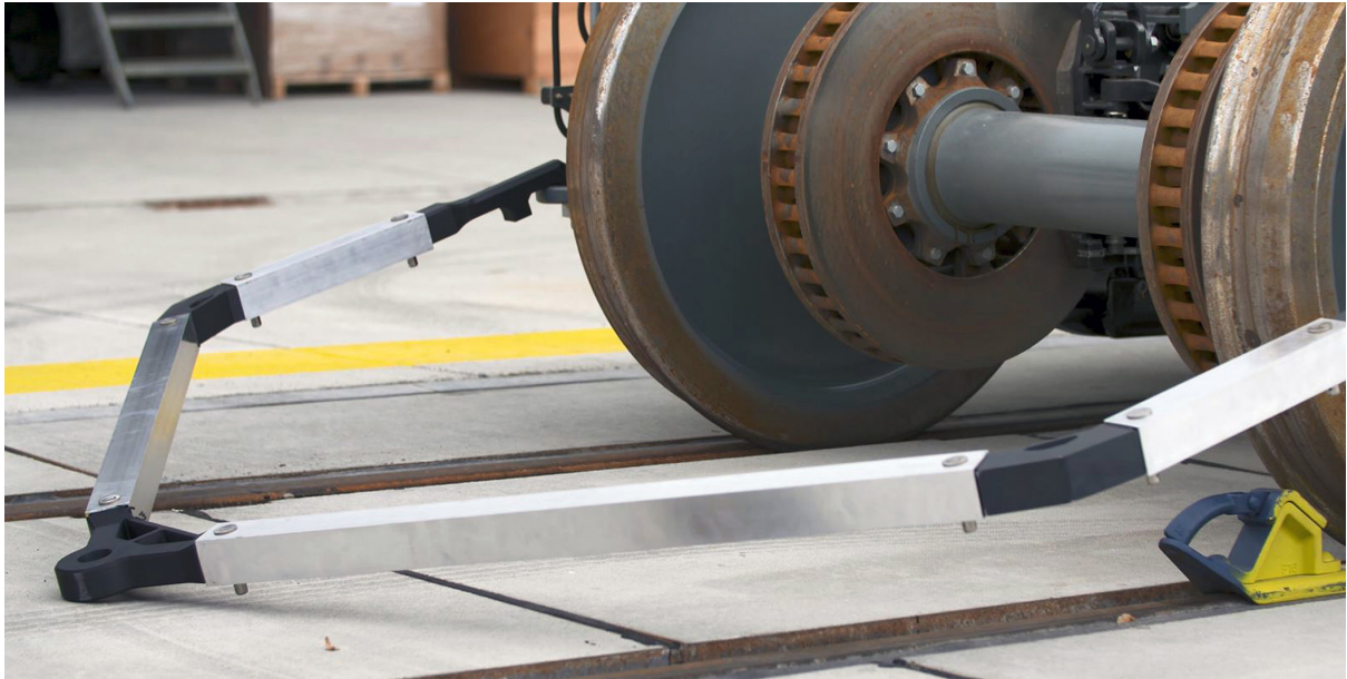
Siemens Mobility is now using its Fortus 450mc to make one-off tools customized to each bogie in a matter of hours.
